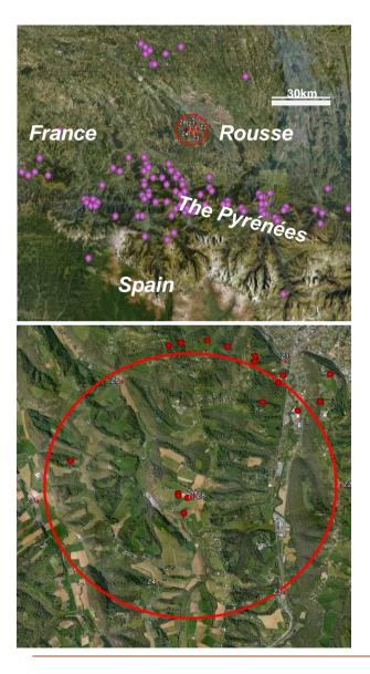
Regional seismicity primarily around the Pyrénées and Lacq depleted gas field
